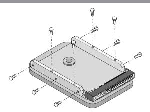
3 Slide the drive carefully into the drive bay. Secure the drive with four 6-32 UNC-2A mounting screws in either the side-mounting holes or the bottom-mounting holes. Do not overtighten the screws. The screws should be inserted no more than 0.22 inch into the bottom mounting holes and no more than 0.14 inch into the side mounting holes. Do not use metric screws.
